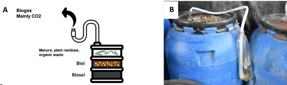
Figure 8: Schematic of a basic design of an on-farm liquid fermentation unit (A). An image of a fermentation vessel in operation in the Andes (B).
