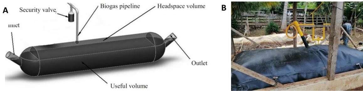
Figure 7: Schematic of a basic design of a tubular-type digester, taken from Garfi et al. (2016) (A). An image of a working tubular digester from <https://www.permaculturenews.org/2020/10/23/biogas-and-carbon-farming-part-3/ml> (B).
